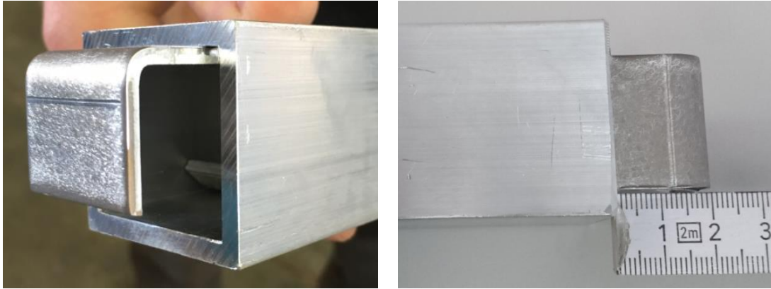
Figure 4: holder within aluminium profile protruding about 20 mm
