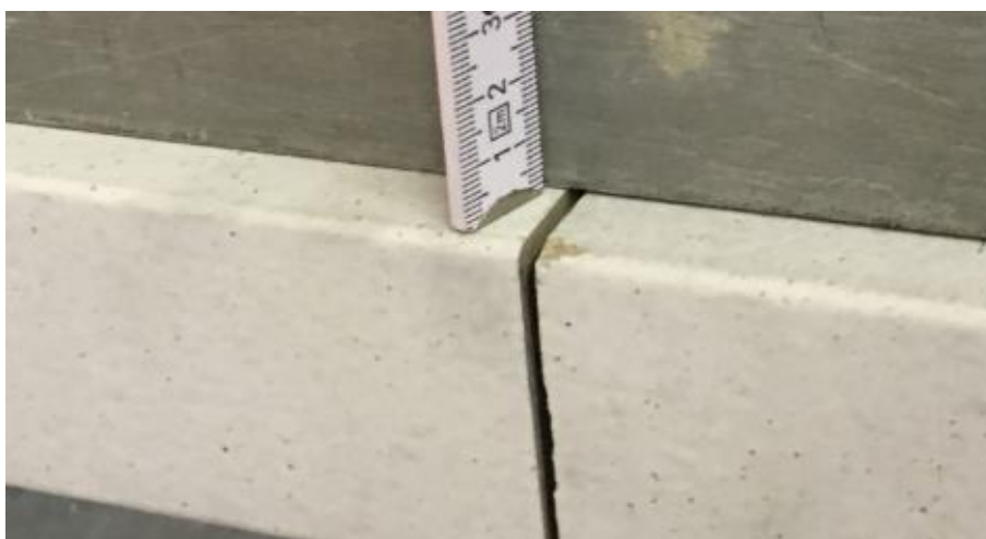
Figure 13: centre deflection caused by dead load less than 1 mm
