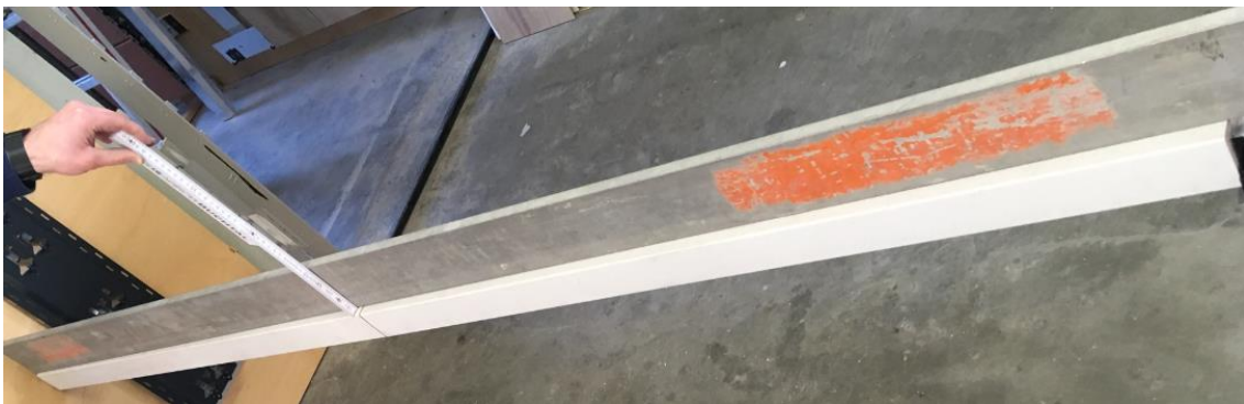
Figure 12: straight edge control of deflection
