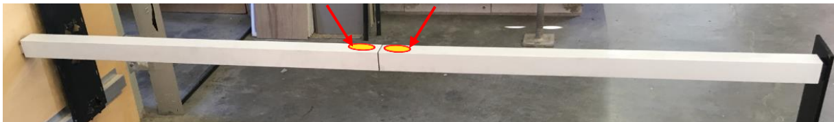
Figure 6: Position of the spring clip at the centre joint on top of the aluminium profile
