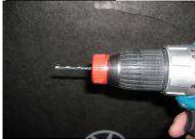
drill bit \varnothing 3,3 mm
