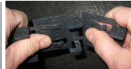
bend the clamp on thread at first to your body and than back, repeat until breakage
