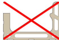
Channel piece with cavities: The result is risks with regard to hygiene, stability and frost resistance (not produced by AGROB BUCHTAL)
